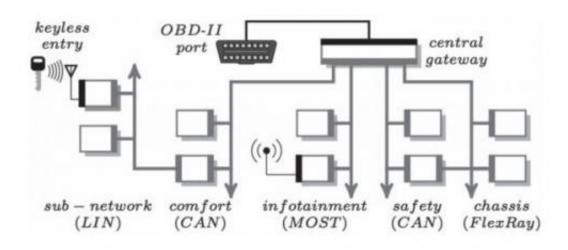
Schematic of a typical in-vehicle network architecture of a modern automobile. Credit: *Intelligent Transportation Systems, IEEE Transactions on*
