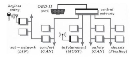
Schematic of a typical in-vehicle network architecture of a modern automobile. Credit: *Intelligent Transportation Systems, IEEE Transactions on*
