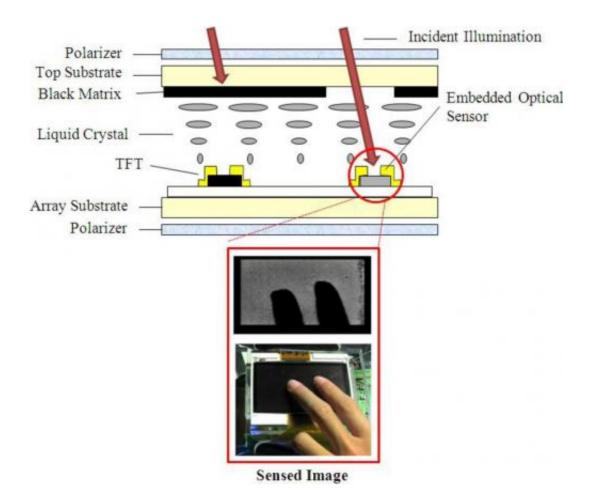
Optical sensors that are embedded in the mobile device detect finger movement. The depth range is currently 3 cm. Credit: Wang, et al. ©2013 IEEE
