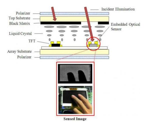
Optical sensors that are embedded in the mobile device detect finger movement. The depth range is currently 3 cm. Credit: Wang, et al. ©2013 IEEE
