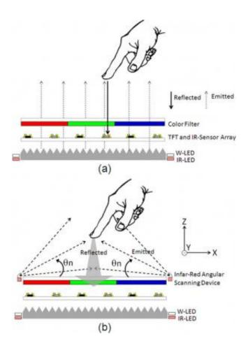
(a) To calculate the 2-axis (x and y) positions of a fingertip, the IR backlight is reflected by the fingertip. (b) To calculate the depth (z) of the fingertip, the system uses IR scanning devices on opposite sides of the display panel. Credit: Wang, et al. ©2013 IEEE
