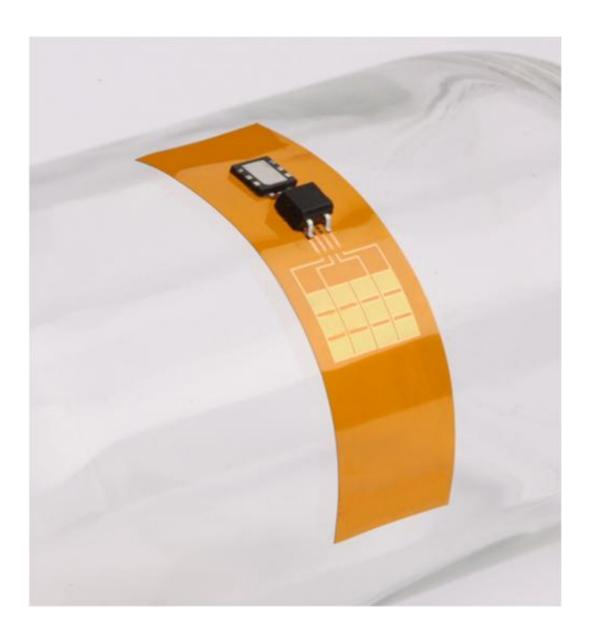
Thin, flexible mechanical energy harvester, with rectifier and microbattery,
