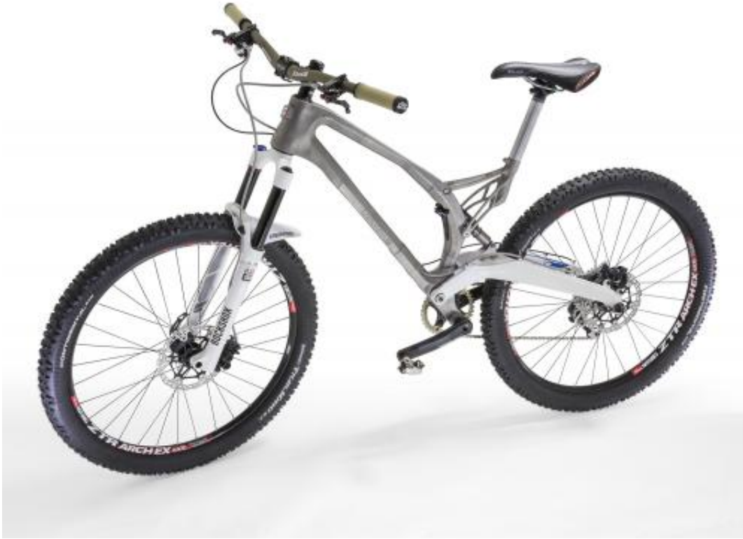
Complete bike with 3D printed titanium alloy frame and seat post bracket
