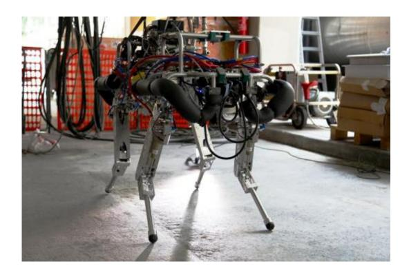
(Phys.org) —HyQ is the latest attention-getter in robotics, a torque-controlled robot that takes its name from its being a "Hydraulically actuated Quadruped." The robot is from the Department of Advanced Robotics at the Istituto Italiano di Tecnologia (Italian Institute of Technology or IIT). A video that demonstrates their progress includes notes that "there are no physical springs in the legs or body of HyQ; all
