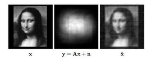
Image sensing and computational reconstruction of Leonardo's Mona Lisa from a lensless phase anti-symmetric spiral phase grating sensor. (Left) The input image. (Middle) The simulated response on the photodetectors due to the six-fold grating, and (right) the reconstruction by. This image estimate is of higher fidelity than the estimate based on traditional square-wave amplitude gratings and photodetector arrays of comparable number of pixels and overall noise level described in earlier work.
