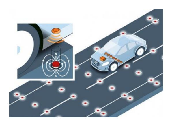
As a potential key to the implementation of self-driving vehicles, Volvo Car Group has completed a research project using magnets in the roadway to help the car determine its position. Incorporating the technology in preventive safety systems could also help prevent run-off road accidents. A pattern of round ferrite magnets (40x15 mm) was located 200 mm below the road surface. The test car was equipped with several magnetic field sensors.
