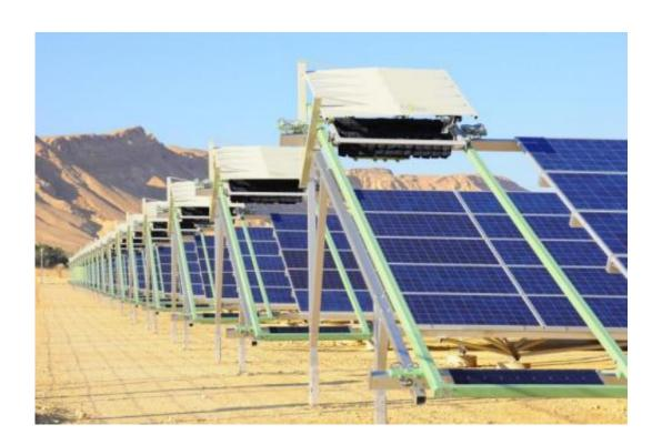
(Phys.org) —At large solar plants, keeping surfaces of solar panels free from dust and sand is not just a matter of good housekeeping but of whether or not the plants can really make a difference to the communities they want to serve. In other words, keeping the panels clean especially in very dry areas may be a matter of solar plant effectiveness or ineffectiveness. Solar plant panels in deserts collect large quantities of
