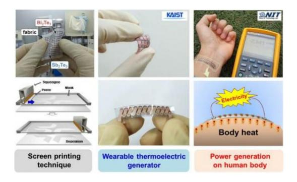
The picture shows a high-performance wearable thermoelectric generator that is extremely flexible and light. Credit: KAIST
