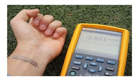
A thermoelectric generator developed as a wristband. The generator can be easily curved along with the shape of human body. Credit: KAIST
