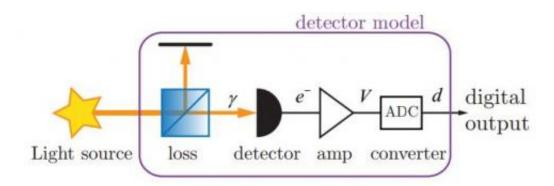
A detector, or indeed each pixel of an image sensor, can be modelled as having 100% efficiency, but being pre- ceded by a lossy element (beamsplitter) with transmission. For each absorbed photon, the detector generates an electron. This charge is then converted into a voltage and amplified, before being digitised and sent to further processing, i.e. a randomness extraction stage. Credit: arXiv:1405.0435 [quant-ph]
