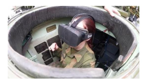
The Norwegian army has announced that they have begun testing the possibility of using the Oculus Rift virtual goggle system in tanks to help expand the field of view for soldiers inside. Such a system would help tank drivers navigate during battlefield operations when the hatch is down, limiting vision for those attempting to maneuver the vehicle during wartime.
