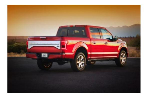
Ford said that the high-strength, military grade, <u>aluminum alloy</u> in the new F-150 does not produce red rust like steel. "We've gone to great lengths to develop coatings that will inhibit corrosion." Also, according to Ford, they standardized the chemistry of the aluminum alloy used in construction of the 2015 F-150 body and bed to facilitate recycling. "Our aluminum scrap can be reclaimed and sent back into the manufacturing process to minimize waste."
