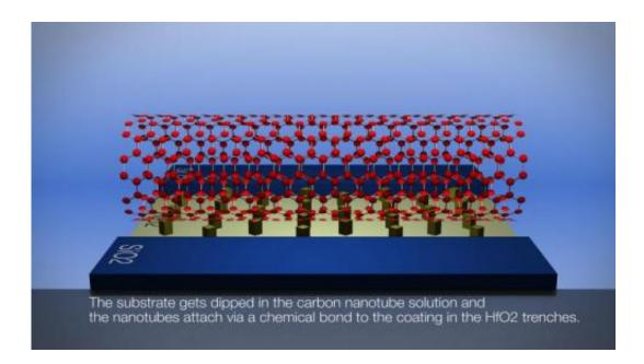
A substrate consists of two oxides - chemically-modified hafnium oxide and silicon oxide. The substrate gets dipped in the carbon nanotube solution and the nanotubes attach via a chemical bond to the coating in the HfO2 trenches. Credit: IBM
