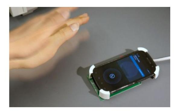
The SideSwipe system. The system leverages the unmodified GSM signal to enable in-air hand gestures both above and on the side of the phone. Credit: Chen Zhao et al.
