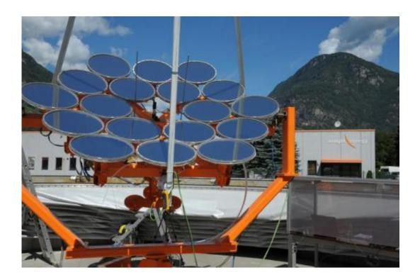
IBM Research and Airlight Energy, a Swiss-based supplier of solar power technology, are bringing a revolutionary, affordable solar technology to the market for sale by 2017. By concentrating the sun's radiation 2,000 times the system can convert 80 percent into useful energy to generate 12 kilowatts of electrical power and 20 kilowatts of heat on a sunny day — enough to power several average\* homes. In this photo a prototype of the system in Biasca, Switzerland at Airlight Energy.
