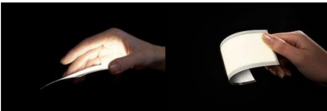
Konica Minolta's flexible OLED panel.
