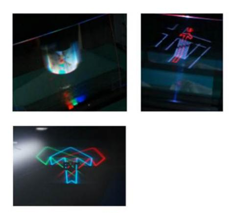
Multiple transparent sheets can be stacked. Credit: Omron/Nikkei Electronics
