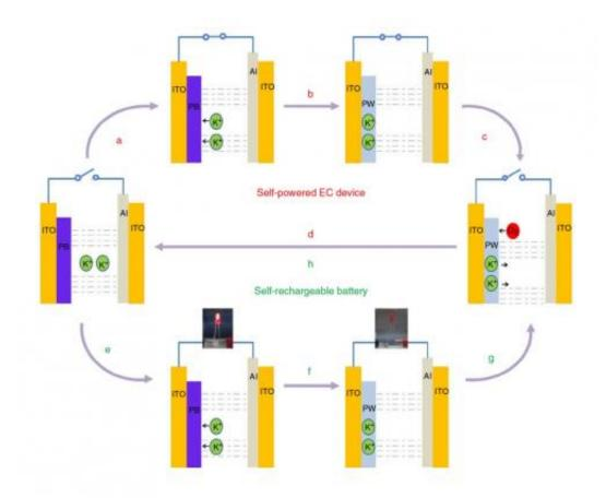
Functioning mechanisms of the bi-functional self-powered EC smart window and self-recharging battery: (a-d) shows the bleaching process of the device serving as a self-powered EC smart window, (e-h) shows the discharging and selfrecharging processes of the device functioning as a self-rechargeable battery. Credit: Wang, et al. ©2014 Macmillan Publishers Limited
