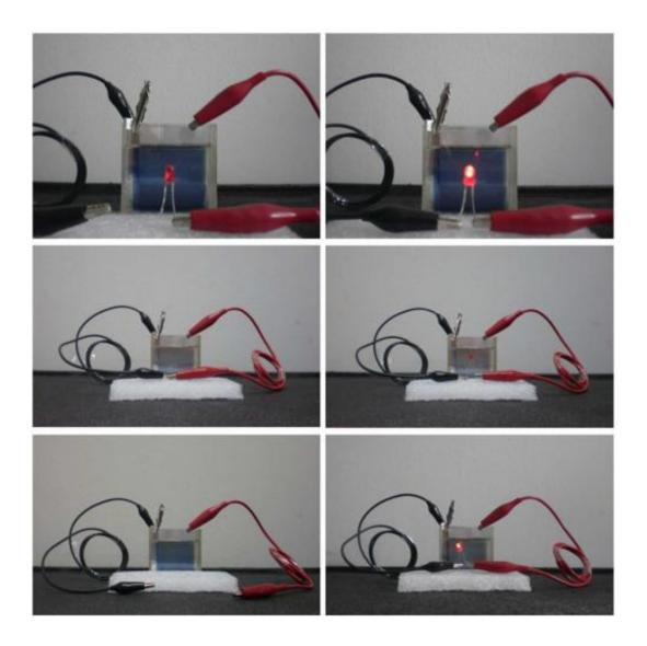
The PB/Al smart window/battery in different states. (a) With the electrodes disconnected, the glass is blue and (b) can power an LED. (c) With electrodes connected, the glass becomes transparent and (d) cannot light the LED. (e) Electrodes are disconnected for one hour to self-recharge the device, and (f) the
