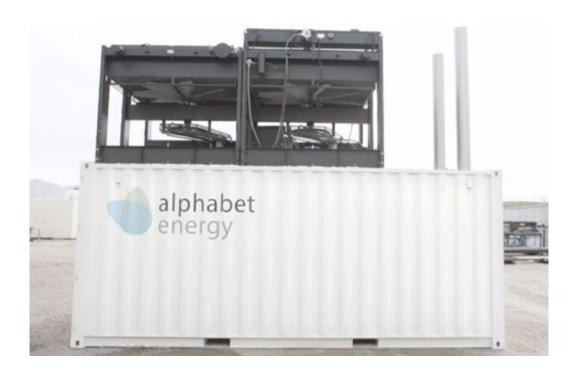
Alphabet Energy has an inexpensive thermoelectric generator, the E1, for waste heat recovery. The generator captures exhaust heat and converts it into electricity. The E1 uses Alphabet's thermoelectric materials to convert the waste heat.
