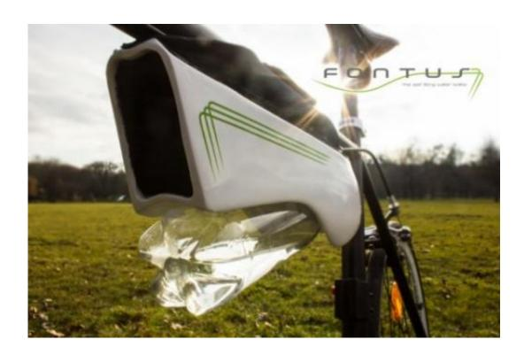
Kristof Retezár, an Austrian designer, has come up with Fontus, which was designed as a self-filling water bottle for your bicycle. This device collects the moisture from the air, condenses it and stores it as safe drinking water. Powered by solar cells, the device harvests up to 0.5 liters in an hour's worth of cycling when under the right climate conditions.
