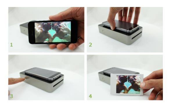
A team of creative types at a small company called Paradigm Optics, with help from a small group of engineers has together created a new way to print pictures taken with a smartphone—and perhaps the best thing about it is that it doesn't require any cables, Bluetooth or even an app on the phone. It's called the SnapJet and to use it, a person calls up a photo on their smartphone, lays the phone on top of the device and then
