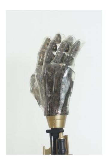
The proposed prosthetic skin conformally attached to the prosthetic hand. The embedded sensor array probides multimodal sensing capabilities corresponding to the actual human skin. Credit: Kim et al.
