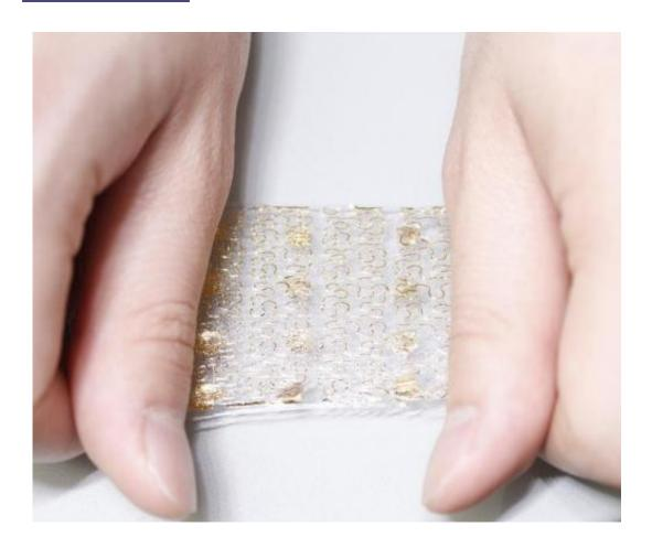
The proposed prosthetic skin is can be stretched freely up to 50%. The embedded sensor arrays are also designed to be stretchable. Credit: Kim et al.
