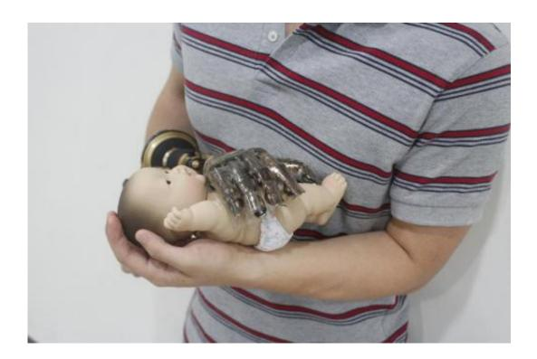
The prosthetic hand equipped with the proposed prosthetic skin is used just like an actual hand to cuddle a baby doll. The prosthetic skin shows soft mechanical properties, multimodal sensing capabilities, and warmth corresponding to that of human body. Credit: Kim et al.
