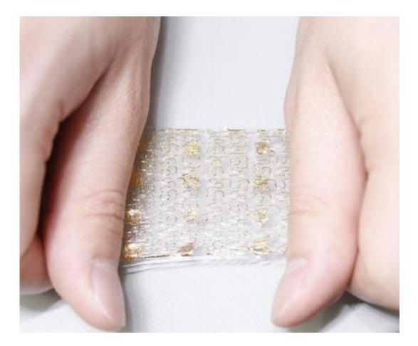
The proposed prosthetic skin is can be stretched freely up to 50%. The embedded sensor arrays are also designed to be stretchable. Credit: Kim et al.
