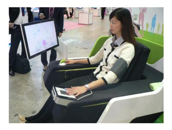
The body weight is measured when the user sits on the equipment. Blood pressure and pulse wave are measured on the left arm and a finger of the right hand, respectively.
