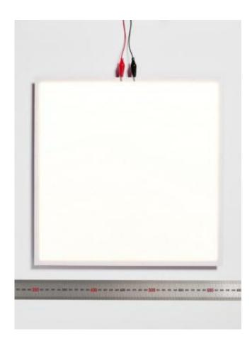
LG Chem is an OLED light panel manufacturer, which provides OLED light panels in various shapes and sizes. Nine models are available with two different color temperatures (3,000K/4,000K), "which deliver high color rendering levels (CRI>90) as well as achieving high luminance,
