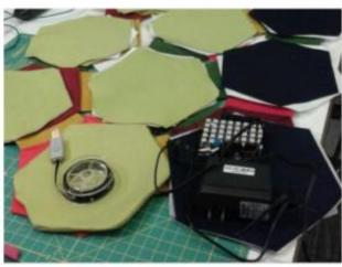
Cotton fabric scarf includes detachable hexagonshaped modules enclosing hardware such as battery-powered vibration modules and heat coil pads. Credit: Michele A. Williams et al.
