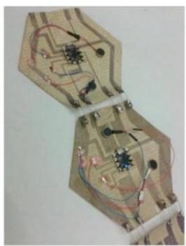
The modular cotton scarf houses canvas modules with conductive fabric circuitry designed to control heat, vibration, and audio actuations. Credit: Michele A. Williams et al.
