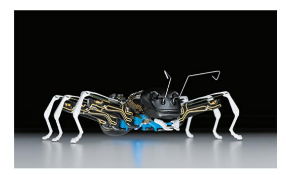
For legs, Festo makes use of piezo technology; they said the bending actuators can be controlled quickly and precisely, work on little energy and do not need much space. Specifically, they use "piezo-ceramic" bending transducers in the legs' actuators.
