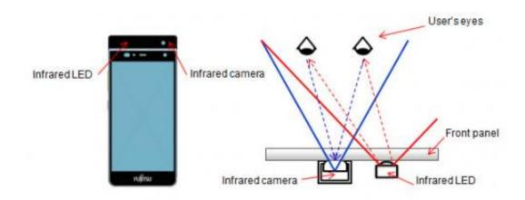
Schematic of smartphone prototype equipped with infrared camera and infrared LED
