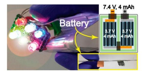
Demonstration of the flexible, 0.5-mm-thick lithium-ion battery being used to light LEDs. Credit: Kim, et al. ©2015 American Chemical Society
