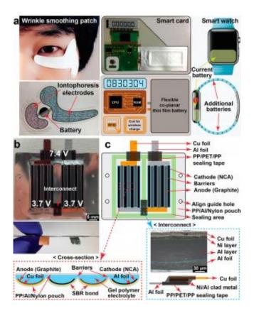
(a) Potential applications of coplanar flexible batteries include a wrinklesmoothing patch, smart card, and smart watch with a supplemental battery in the watch strap. (b) Photographs and (c) illustrations of the battery. Credit: Kim, et al. ©2015 American Chemical Society
