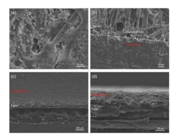
SEM images of a) unmodified printing paper and b) part of pencil-trace drawn on the paper. c) 45° Side view and d) cross-sectional image of the paper coated with graphite film. Credit: *Advanced Functional Materials*,
