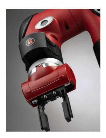
Sawyer is a new collaborative robot (robots that work with employees) from Boston, Massachusetts-based Rethink Robotics. In human terms, the salient feature about this robot is its friendly eyes on its "face" screen. On the technical side, the salient feature is its single arm designed to execute machine-tending, circuit-board testing and other
