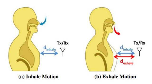
Chest Motion Changes the Signal Reflection Time. (a) shows that when the person inhales, his chest expands and becomes closer to the antenna, hence decreasing the time it takes the signal to reflect back to the device. (b) shows that when the person exhales, his chest contracts and moves away from the antenna, hence the distance between the chest and the antenna increases, causing an increase in the reflection time. Credit: Fadel Adib et al.
