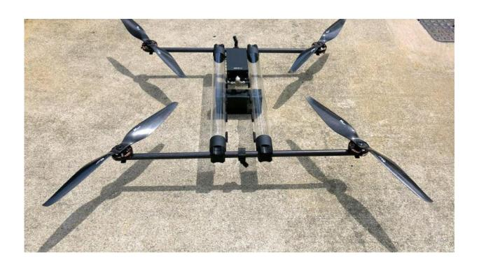
Singapore-based Horizon Unmanned Systems (HUS) this month introduced the hycopter, which they said is the world's first hydrogen fuel cell-powered multi-rotor UAV. It uses refillable hydrogen tubes as part of its structure.
