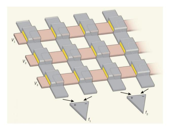
A memristive neural network. The cartoon depicts a fragment of Prezioso and colleagues' artificial neural network, which consists of crossing horizontal and vertical wires that have memristor devices (yellow) at the junctions. Input voltages V1 to V3 (the network inputs) drive currents through the memristors, and these currents are summed up in the vertical wires. Artificial neurons (triangles) process the difference between currents in neighbouring wires to
