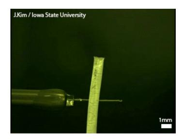
This movie shows the soft-robotic micro-tentacle's grabbing and releasing motion dynamically in real-time. The target is a thread of dental floss. (Scale bar: 1 mm). Credit: Jaeyoun Kim / Iowa State University
