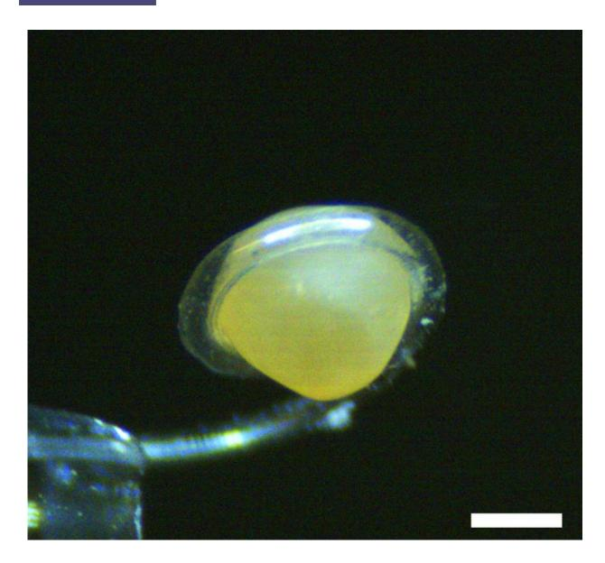
The soft-robotic micro-tentacle is "scooping up" the fragile fish egg using its conformally wrapped arm as the support. (Scale bar: 0.5 mm). Credit: Jaeyoun Kim / Iowa State University
