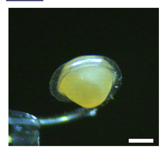
The soft-robotic micro-tentacle is "scooping up" the fragile fish egg using its conformally wrapped arm as the support. (Scale bar: 0.5 mm). Credit: Jaeyoun Kim / Iowa State University
