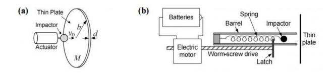
Conceptual sketches of: (a) impact transmitter; and (b) electromechanical pull-type actuator. Credit: arXiv:1507.01479 [physics.ins-det]
