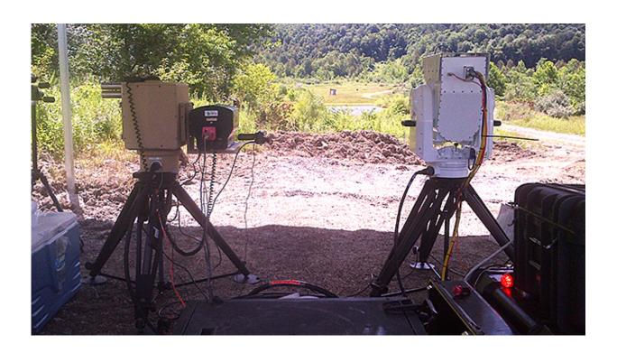
Consider a contest of unmanned aerial vehicle versus energy. And one where energy wins. Boeing has a compact laser weapons system to pull the win off. The system directs energy on its targets, focusing energy on a spot in order to damage the target. Think of it as a welding torch, said Isaac Neal, Boeing engineer, but from many hundreds of meters away.
