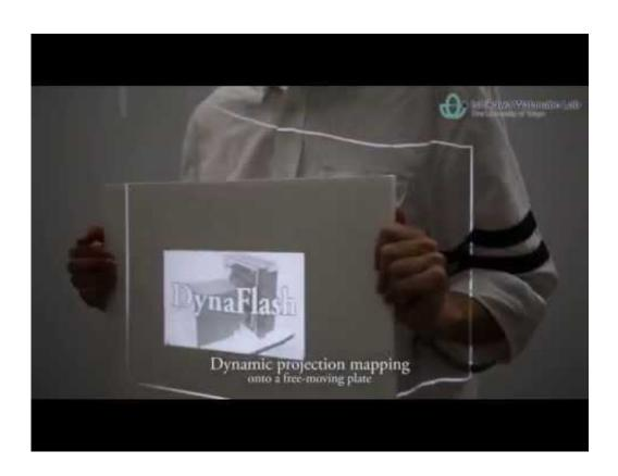
A team from the Ishikawa Watanabe Laboratory at Tokyo University and Tokyo Electron Device (TED) have come up with a prototype of a high-speed projector called "DynaFlash" which can project 8-bit images up to 1,000fps with 3ms delay. DynaFlash is actually a projection mapping system for tracking objects moving at high speed. A video
