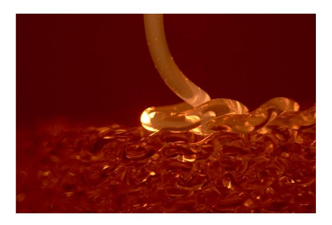
Fine glass manufactured additively has been the focus of a team of MIT researchers, who demonstrate their new method of making glass via advanced 3D printing.
