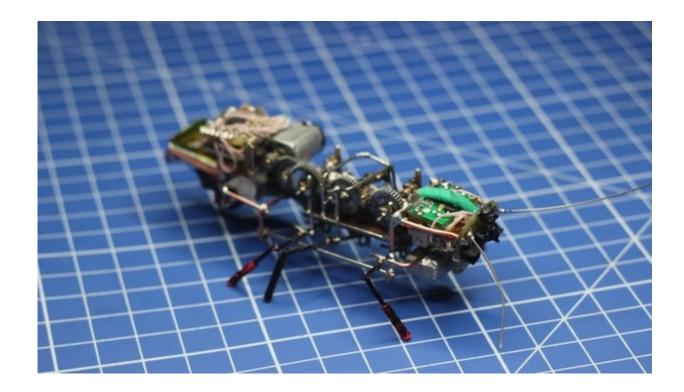
Earlier this year, engineers in Texas worked on a robotic insect fusing a real cockroach with a miniature <u>computer</u> wired into the animal's nervous system, said *The Guardian*. At the push of a button, a human operator can control which way it scuttles.
