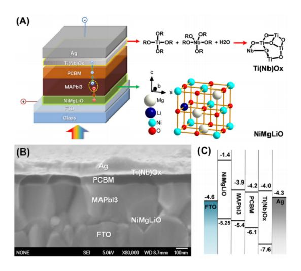
Structure and band alignments of the PSC. (A) Scheme of the cell configuration highlighting the doped charge carrier extraction layers. The right insets shows the composition of Ti(Nb)Ox and the crystal structure of lithium doped NixMg1-xO, denoted as NiMg(Li)O. (B) A high resolution cross– sectional SEM image of a complete solar cell (the corresponding EDX analysis results are
