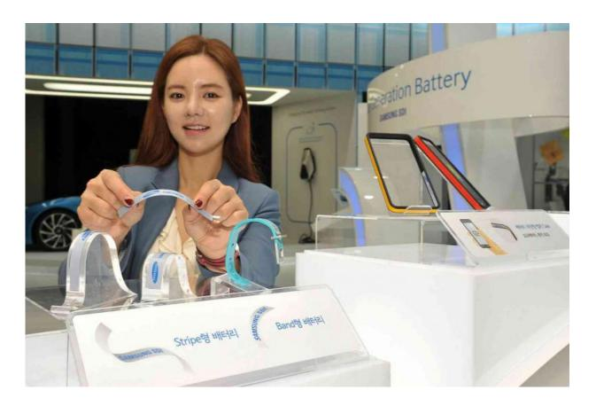
Meanwhile, the Stripe Battery is described as slim and flexible with highenergy density. This one can be adapted to any wearable such as necklace, hairband and T-shirts. It bends and conforms freely as a fiber.
