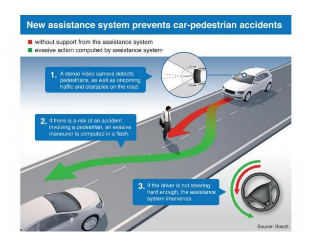
New assistance system prevents car-pedestrian accidents. If there is a risk of an accident involving a pedestrian, an evasive maneuver is computed in a flash. If the driver is not steering hard enough, the assistance system intervenes.
