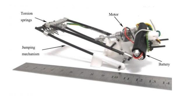
Prototype of TAUB, the 23-gram miniature jumping robot. Credit: Zaitsev, et al. ©2015 IOP Publishing Ltd
