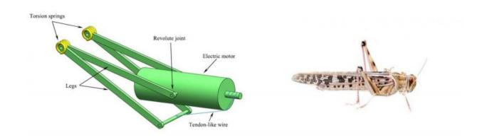
Conceptual design of the robot compared to a desert locust. Credit: Zaitsev, et al. ©2015 IOP Publishing Ltd
