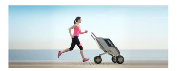
Smartbe is the name of an intelligent stroller, intelligent in the way it deploys a motion tracking sensor system and follows the stroller's parent or caregiver. The stroller can follow when the person walks, <u>stops</u>, steps backwards, or continues walking forward.
