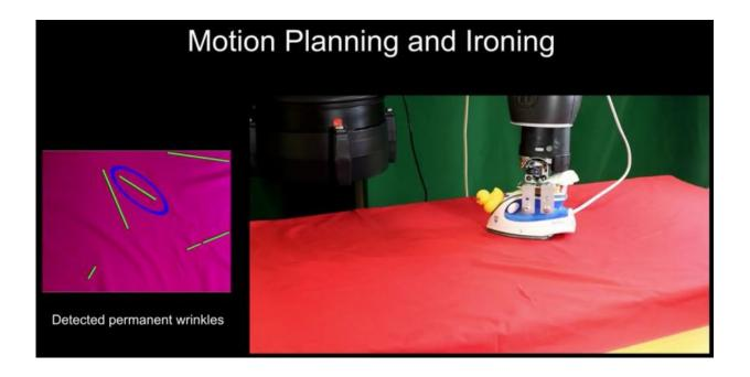
Can a piece of cloth be properly ironed autonomously? Can a robot handle a regular iron and remove wrinkles?
