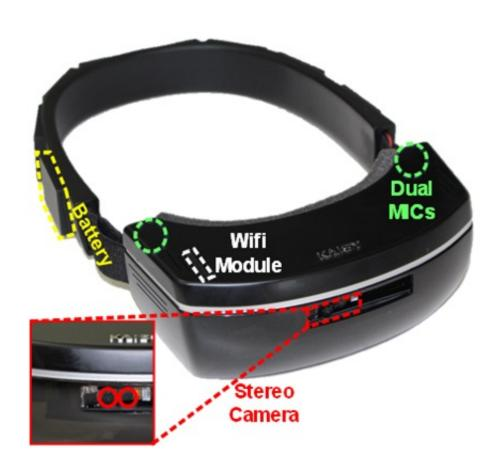
K-Glass 3 is equipped with a stereo camera, dual microphones, a Wi-Fi module, and eight batteries to offer higher recognition accuracy and enhanced augmented reality experiences than previous models. Credit: KAIST
