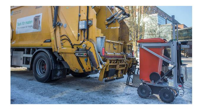
When it is time to begin waste collection, the driver of the refuse truck presses a button. This starts the robot and the drone simultaneously lifts from the roof of the truck. Flying through alleyways, the drone quickly finds the location of the refuse bins and communicates their positions to the robot. This is followed by automatic waste collection and emptying by the robot. In the cab, the driver is able to monitor the exact location of the <u>robot</u> and the emptying process.
