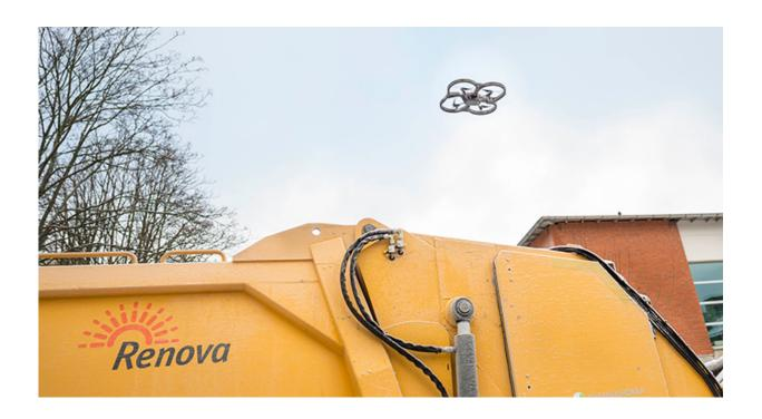
Students from three universities have collaborated with the Volvo Group and the waste recycling company, Renova. The result is a robot that automatically collects and empties refuse bins. A drone on the roof of the refuse truck scans the area and helps the robot to find the bins.
