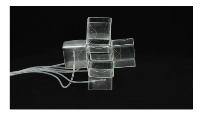
Harvard researchers have designed a new type of foldable material that is versatile, tunable and self actuated. Here a single cell is folds according to its actuation. Credit: Johannes Overvelde/SEAS
