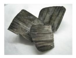
Lithium ingots with a thin layer of black oxide tarnish. Image: Wikimedia Commons
