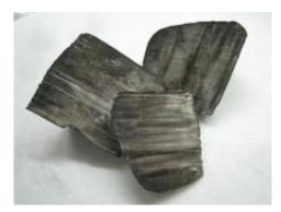
Lithium ingots with a thin layer of black oxide tarnish. Image: Wikimedia Commons
