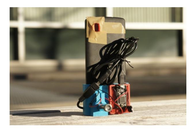
The researchers prototyped the sensor using the camera in an ordinary cellphone and a commodity laser emitter that costs about \$10.
